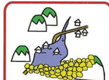
Natural damming of river caused by landslides → Collapse → Debris flow
